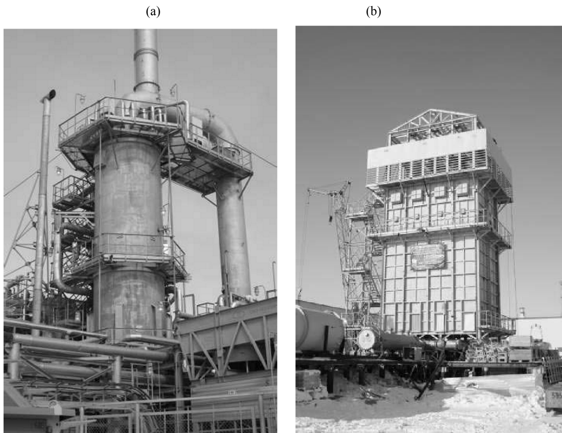
Fig. 5. (a) Cylindrical and (b) box-shaped (“Penthouse” type) reformers available from Metaprotsess Closed Joint-Stock Company, installed at mineral resources user’s site beyond the Arctic Circle: reaction temperature 850°C; number of tubes: (a) 26 and (b) 48; number of burners: (a) 7 + 3 and (b) 32 + 8; gas capacity: (a) 2200 and (b) 7500 \text{Nm}^3 \text{h}^{-1} ; and congas capacity: (a) 7900 and (b) 27300 \text{Nm}^3 \text{h}^{-1} .
